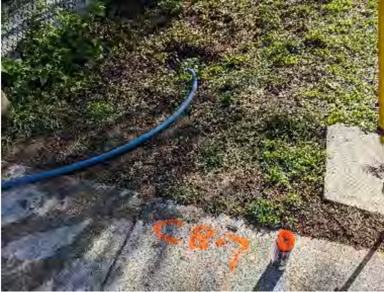
14. CB-7 on Campbell connects to COMB-D (green dye)
